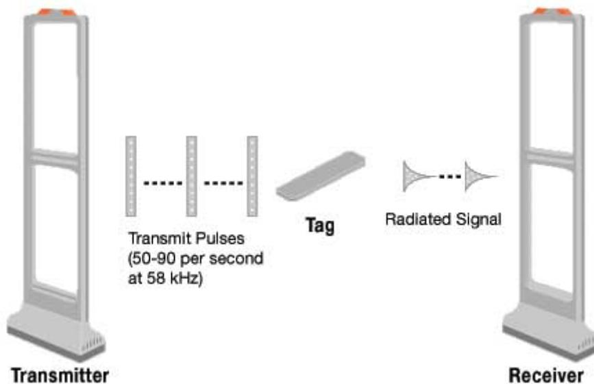
AM material is highly **magnetostrictive**, which means that when you put the tag material in a magnetic field, it physically shrinks. The higher the magnetic field strength the smaller the metal becomes. The metal actually shrinks about one-thousandth of an inch over its full 1.50 inch length.
